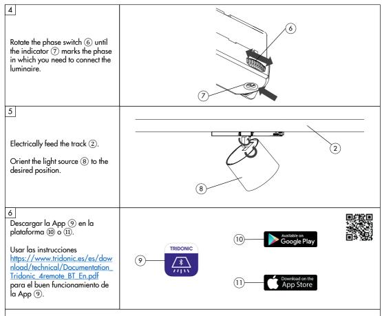
**NOTE**: To move the luminaire on the electrified track or to change the phase, previously make sure that the track has not network voltage.
